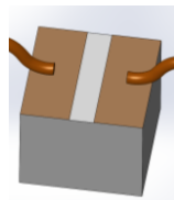
Capacitor (250 \mu m x 200 \mu m x 250 \mu m)
